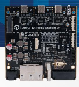
DSBOARD-ORNX-LAN is an industrial carrier board designed for harsh environments and applications that demand high processing power and reliability. It is based on the NVIDIA Orin NX system-on-module (SOM), which features multiple NVIDIA Ampere GPU cores and Arm64 CPU cores. The compact design of the carrier board makes it a versatile and flexible solution for a wide range of industrial applications such as autonomous systems, robotics, and intelligent video analytics.
