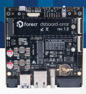
DSBOARD-ORNX is an industrial carrier board designed for harsh environments and applications that demand high processing power and reliability. It is based on the NVIDIA Orin NX system-on-module (SOM), which features multiple NVIDIA Ampere GPU cores and ARM64 CPU cores. The compact design of the carrier board makes it a versatile and flexible solution for a wide range of industrial applications such as autonomous systems, robotics, and intelligent video analytics.
