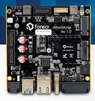
DSBOARD-AGX is a powerful and reliable edge computing device designed for industrial applications that require high processing power and ruggedness. It is based on the NVIDIA Jetson AGX Orin systemon-module (SOM), which features an NVIDIA Ampere GPU with 1024 CUDA cores and up to 275 TOPS (trillion operations per second) of Al performance. The AGX Orin SOM also includes a 12-core ARMv8.2 CPU and a dedicated deep learning accelerator for efficient inferencing.
